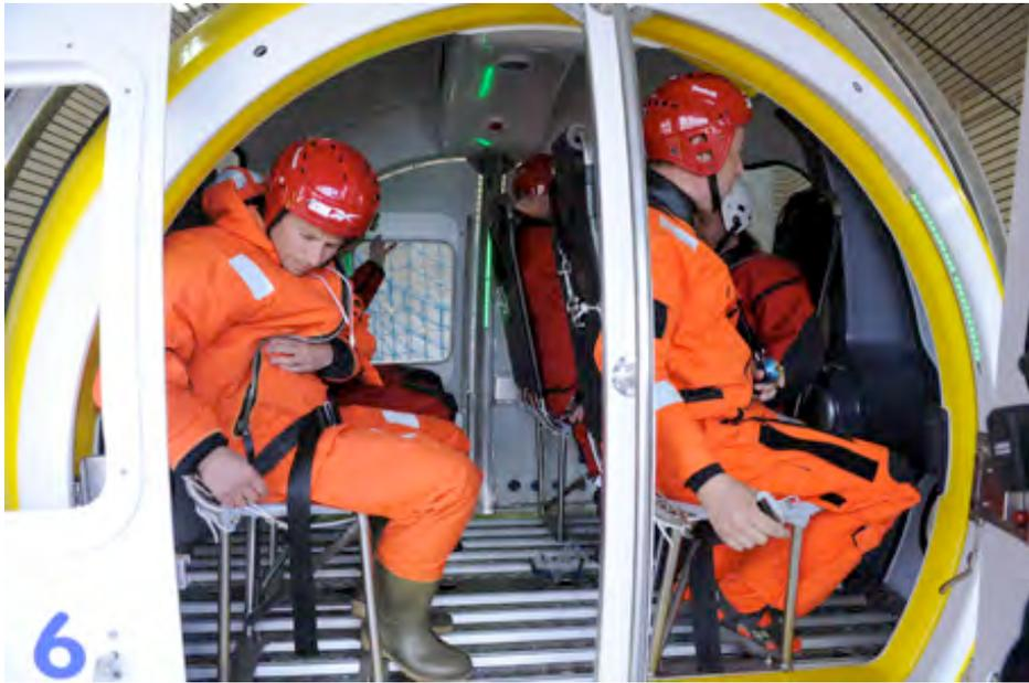
*The participants strap themselves in and give the go-ahead to the instructor. A video camera with a wide-angle lens, which is mounted in the ceiling of the MWH, records what happens during the drill. The film sequences are used in the theoretical section of the training program and can also be used in an evaluation of the drills. The “green lines” are emergency exit lighting.*
