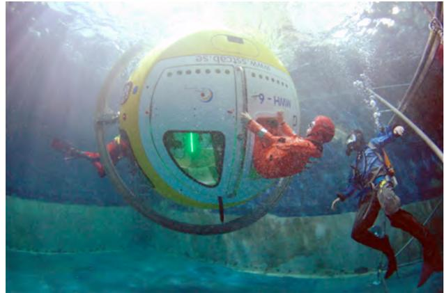
*The difficulty of the drills is gradually increased and the cabin is allowed to rotate and fill with water before evacuation takes place via doors that are opened in the normal way or with an emergency handle, or via removable windows. To guarantee safety, there are always safety divers in the water who can provide air and help.*
