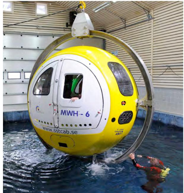
*The crane operator plays an important role in the safety aspects of the drills. He guides the MWH to the position where it is to be launched. The ballast tanks are filled and emptied via a remote control.*
