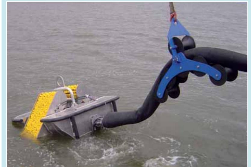
The Lamor Free Floating Offshore skimmer is a very high capacity free-floating skimmer designed for open ocean oil recovery operations. The LFF 100 2C is fitted with two V-chain-pocket-brush conveyors for efficient collection of all types of floating oil, from light to high viscosity oils, emulsion and bitumen as well as debris-laden oil.
